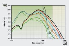
ABOVE: Nearfield driver (solid) & port (dashed) resp. for the LōKē with LPF at 120Hz, black; 100Hz, red; 80Hz, blue; 60Hz, orange; 40Hz, green (all 12dB/oct)
